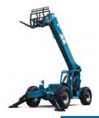
Audible back-up travel alarm mounted in counterweight area signals reverse movement.
